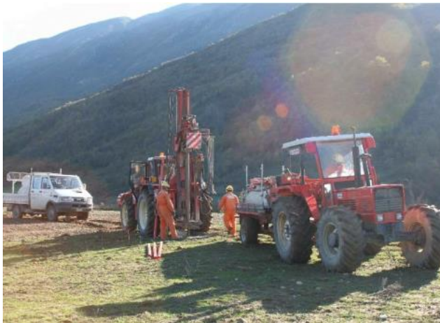
Figure 2-7 Example of Tractor mounted drill rig
