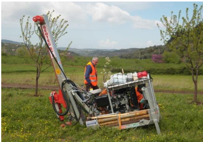
Figure 2-8 Examples of heli-portable drill rigs
