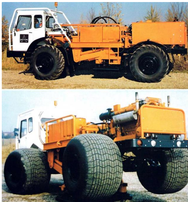
Figure 2-10 Example of a vibroseis truck
