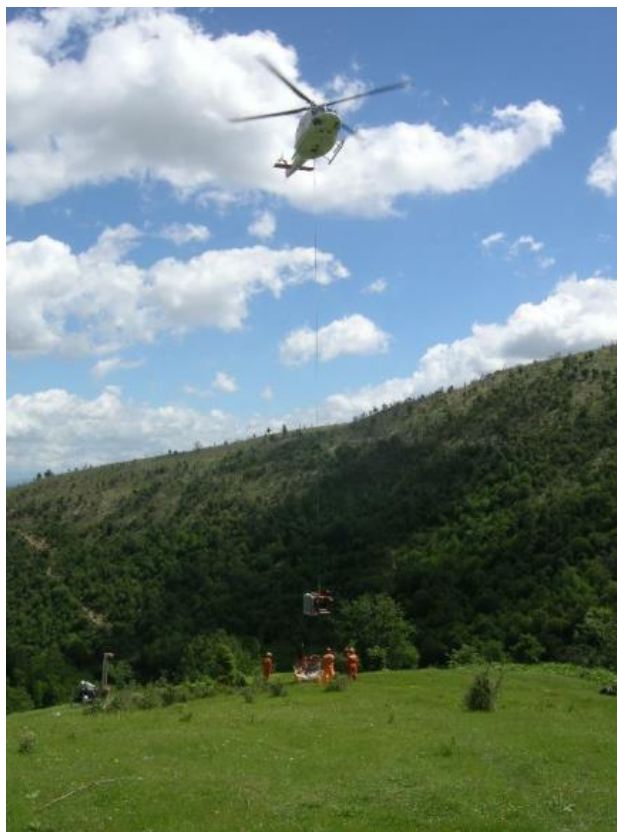
Figure 2-12 Example of a helicopter transporting a drill rig
